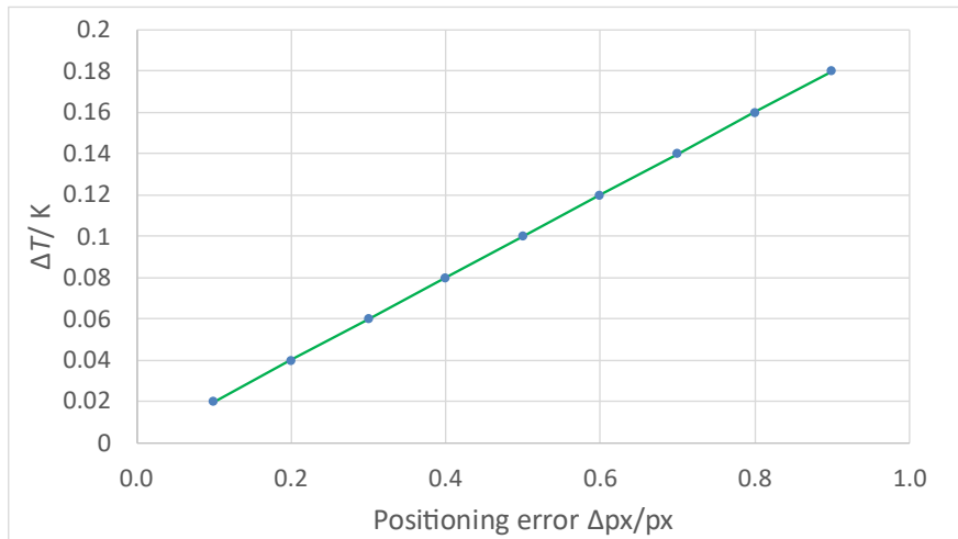
Figure 1 Simulated influence of the positioning accuracy assuming a blackbody at 100 °C in compliance with VDI/VDE 3511 Blatt 4.6 [2] and a maximum non-uniformity of the radiation temperature of \pm 0.2 K.
