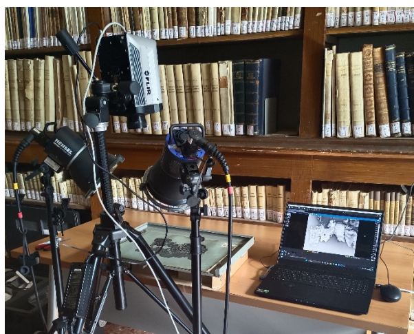
Figure 2. PT setup in situ during the acquisition on papyri fragments.
